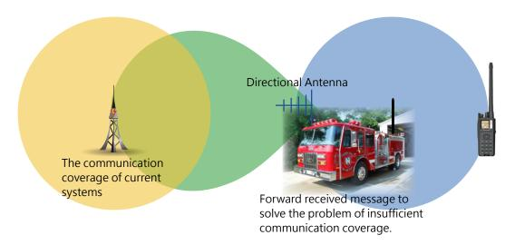
When users are out of the communication range covered by the systems, or the current system is damaged or malfunctioning, BR02 can quickly extend the communication range.
