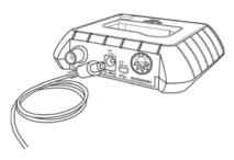
Step 1. Connect the power cable to the E5 charger power socket. Step 2. Plug the AC transformer into a wall outlet.
