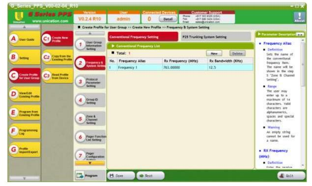
II. To build your P25 trunking system you must select the grey tab at the top that says P25 Trunking System Setting. The information that you will need is the systems WACN ID, The System ID, the RFSS ID and Site ID's for each site along with the control channels for those sites. This information should be obtained through your system admin.
