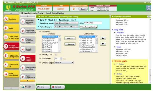
XI. The Unmute Logic on a Multichannel scan must be set to Match ID in order for the PL tones to work.
